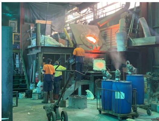
Photo #2 – Molten metal ready for discharge into distribution crucible
