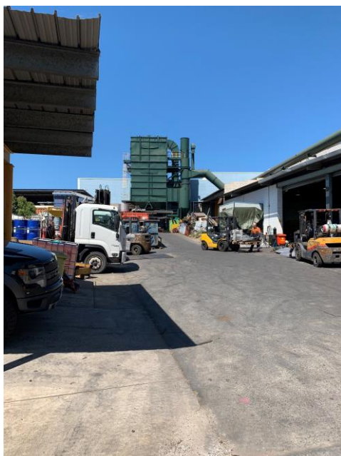
Photo #1 – Reverse pulse type dust collector at eastern end of Clingcast site
